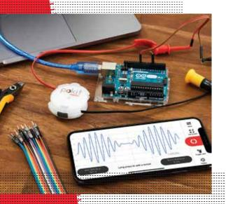
Pokit Meter measures, displays and logs a wide range of parameters including voltage, current, resistance and temperature. It also provides a continuity and diode checker.
