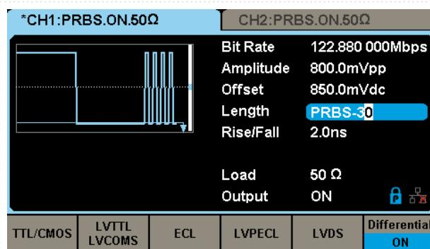
Preset common logic levels such as TTL, LVCOS, LVPECL and LVDS. An added differential mode provides an easy way to generate differential signals using the both channels.
