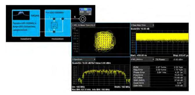
The SDG7000A can generate common modulation types of IQ signals, such as ASK, FSK, PSK, QAM. With the innovative resampling technology, excellent EVM performance can be obtained at any symbol rate between 250 S/s ~ 500 MS/s. The built-in digital quadrature modulator can modulate the carrier of the IQ signal to any frequency between 0 Hz~1 GHz. The EasyIQ software can be used to generate and edit various types of IQ signals.
