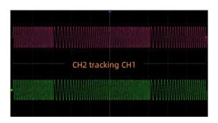
**Track/Copy/Coupling** The track, copy and coupling functions between the two channels can quickly transfer the parameters of one channel to the other according to the requirements, greatly simplify the operation and meet the requirements of fast and synchronous switching waveforms.
