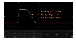
**Flexible edge** Adjustable fine step resolution to 100 ps. The minimum edge is 500 ps and can be generated at any frequency. The rising/ falling edge can be set respectively and can be used to generate asymmetric pulse
