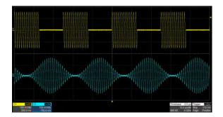
**Modulation** A variety of analog and digital modulation modes such as AM, FM, PM, FSK, ASK, PSK, DSB-SC, and PWM are supported. There are three modulation sources: Internal, External, and Channel.
