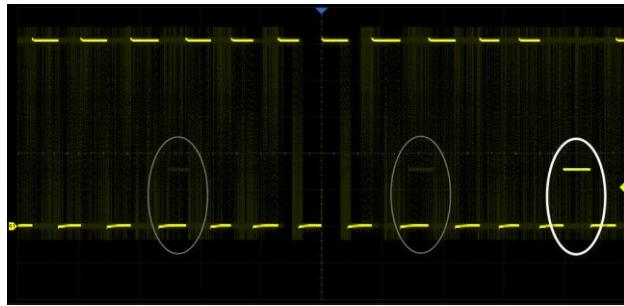
With a waveform update rate of up to 160,000 wfm/s, the oscilloscope can easily capture unusual or low-probability events. In Sequence mode, the waveform capture rate can reach 650,000 wfm/s
