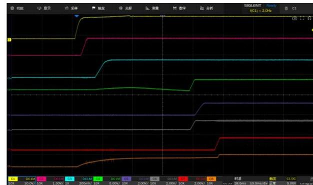
The oscilloscopes can capture the power-on process of up to 8 signals at one time, saving measurement time, improving work efficiency, reducing errors introduced by multiple measurements
