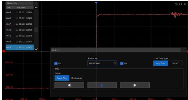
History function can record up to 170,000 frames of waveforms. The recording is executed automatically so that the customer can playback the history waveforms at any time to observe unusual events and quickly locate the area of interest using the cursors or measurements. The failed frames of the Mask Test can be stored as history
