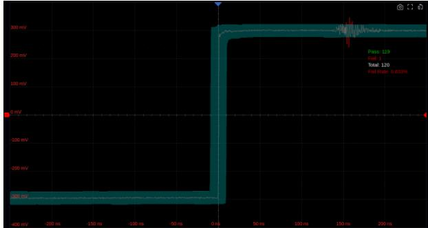
The oscilloscope utilizes a hardware-based Mask Test function, performing up to 28,000 Pass / Fail decisions each second. It is easy to generate user-defined test templates to provide trace mask comparisons, making it suitable for long-term signal monitoring or automated production line testing
