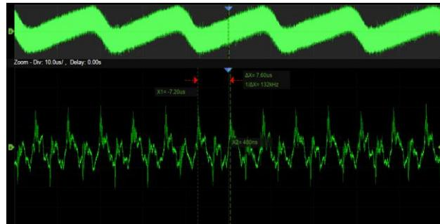
Using hardware-based Zoom technique and record length of up to 2.5 Gpts, users can select a slower timebase without compromising the sample rate, and then quickly zoom in to focus on the area of interest
