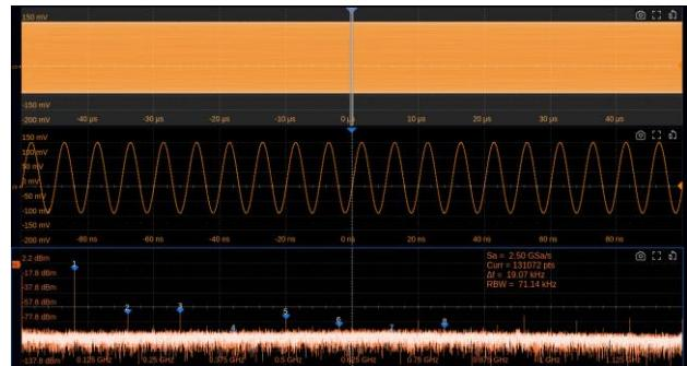
FFT supports up to 8 Mpts operation. This provides high-frequency resolution with a fast refresh rate. The FFT function also supports a variety of window functions so that it can adapt to different spectrum measurement needs. Three modes (Normal, Average, and Max hold) can satisfy different requirements for observing the power spectrum. Auto peak detection and markers are supported.
