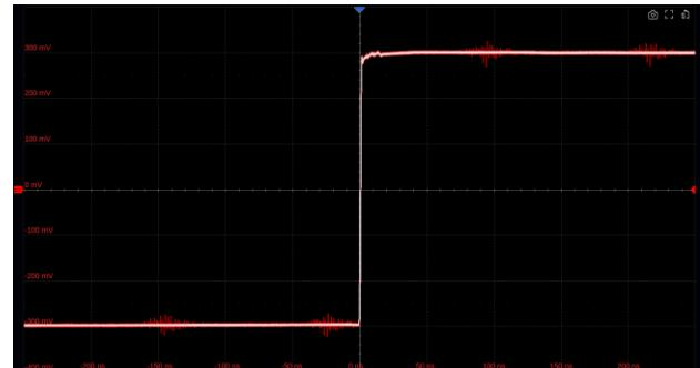
Segmented memory collection will store the waveform into multiple memory segments (up to 170,000) and each segment will store a triggered waveform as well the dead time information. The interval between segments can be as small as 1.5  $\mu$ s. All of the segments can be played back using the History function
