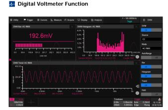
4-digit voltmeter and 7-digit frequency counter. Any analog channel can be selected as a source. Bar, Histogram and Trend diagrams are supported
