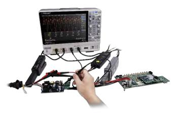
The Power Analysis option provides a full suite of power measurements and analysis, which greatly improve the measurement efficiency in switching power supplies and power devices design
