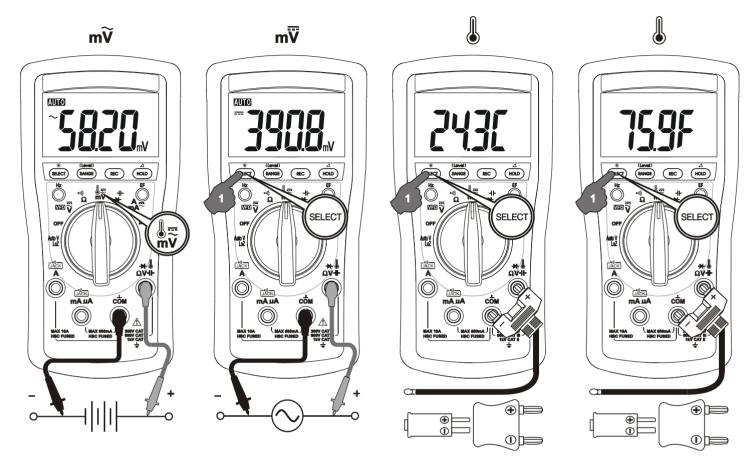
Note: Be sure to insert the banana plug type-K temperature bead probe Bkp60 with correct + – polarities. You can also use a plug adapter Bkb32 (Optional purchase) with banana pins to type-K socket to adapt other standard type-K mini plug temperature probes.
