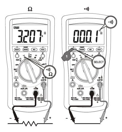
→) BeepLit<sup>TM</sup> Continuity function is having improved convenience for checking wiring connections and operation of switches. A continuous beep tone together with flashing display backlight indicate a complete wire. Such audible and visible indications improve continuity readabilities in noisy working environments.
