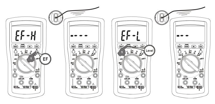
•*Non-Contact EF-Detection*: An antenna is located along the top-left end of the meter, which detects electric field surrounding energized live conductors. It is ideal for tracing live wiring connections, locating wiring breakages and to distinguish between live and earth connections.
