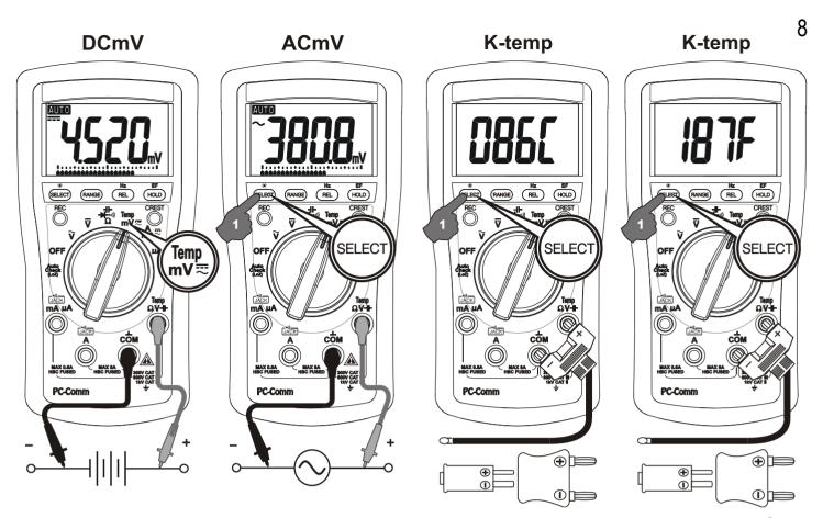
Note: Be sure to insert the banana plug K-type temperature bead probe Bkp60 with correct **+ –** polarities. You can also use a plug adapter Bkb32 (Optional purchase) with banana pins to K-type socket to adapt other standard K type mini plug temperature probes.
