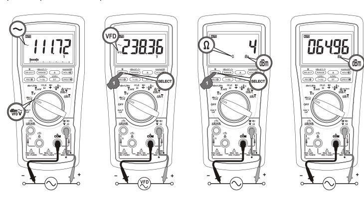
**Note:** In **dBm** function, power up default reference impedance will be displayed for 1 second before displaying the dBm readings. Press **dBm-\Omega** (**RANGE**) button momentary to select different reference impedance of 4, 8, 16, 32, 50, 75, 93, 110, 125, 135, 150, 200, 250, 300, 500, 600, 800, 900, 1000, up to 1200 $\Omega$ . Last selection will be saved as power up default for repeat measurement convenience.
