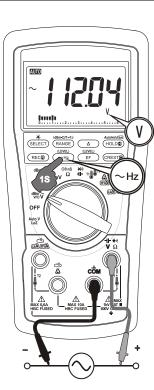
**Note:** It is recommended to direct measure the signals (voltage or current) in autoranging mode before activating the ~Hz function right in that range to get the most appropriate trigger level automatically. If the ~Hz reading is unstable, select lower sensitivity to avoid possible electrical noises. If the reading shows zero, select higher sensitivity to measure.
