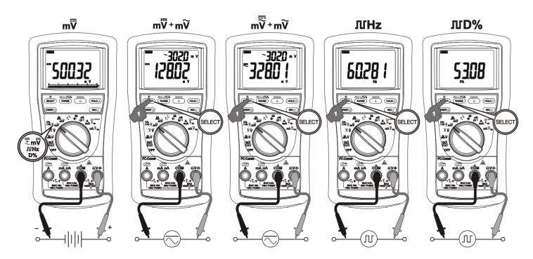
ACmV +Hz, dBm +Hz, Hz +ACmV functions
