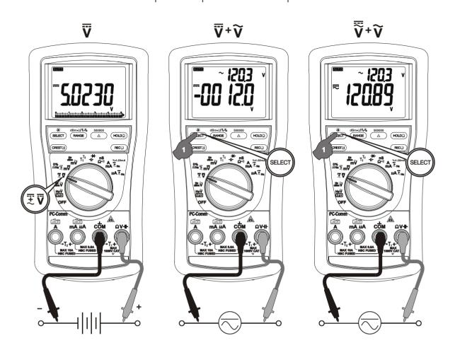
DCmV, DCmV +ACmV, DC+ACmV +ACmV, Logic-Level **11** Hz, Duty% functions Press the SELECT button momentarily to select the subject functions in sequence. Last selection will be saved as power up default for repeat measurement convenience.
