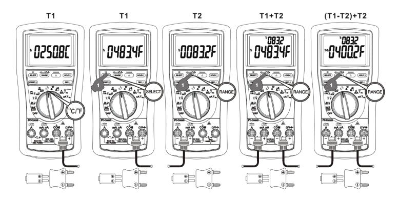
Note: Be sure to insert the banana plug type-K temperature bead probe Bkp60 with correct + polarities. You can also use a plug adapter Bkb32 (Optional purchase)
