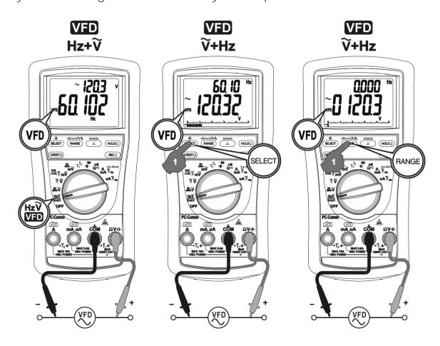
Note: Hz Input sensitivity varies automatically with voltage (current function alike) range selected. 5V range has the highest and the 1000V range has the lowest. This VFD function defaults at the most appropriate trigger level for Variable Frequency
