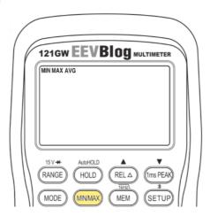
To find the minimum and maximum value found during sampling you can use the MIN/MAX button.
