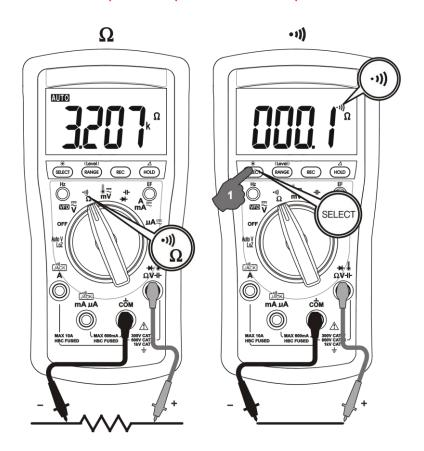
• )BeepLit™ Continuity function is having improved convenience for checking wiring connections and operation of switches. A continuous beep tone together with flashing display backlight indicate a complete wire. Such audible and visible indications improve continuity readabilities in noisy working environments.
