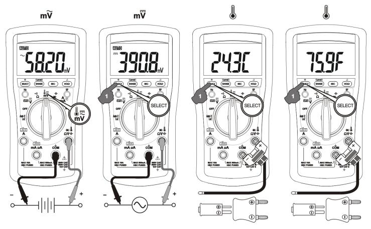
Note: Be sure to insert the banana plug type-K temperature bead probe Bkp60 with correct Xpolarities. You can also use a plug adapter Bkb32 (Optional purchase) with banana pins to type-K socket to adapt other standard type-K mini plug temperature probes.
