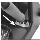
Place the handpiece in the extractor and pull to remove the cartridge.
