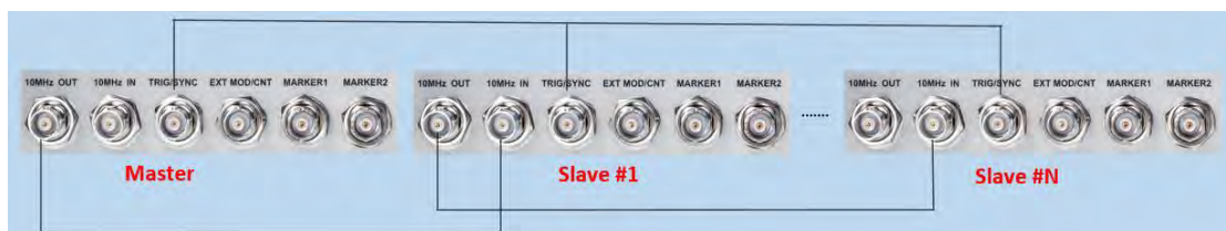
Figure 17-1 wiring diagram of multi-device synchronization
