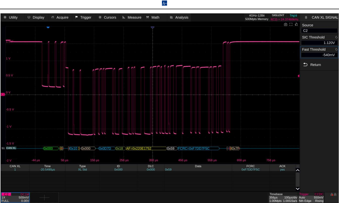
Figure 7 CAN XL Fast Mode Protocol signal Settings
