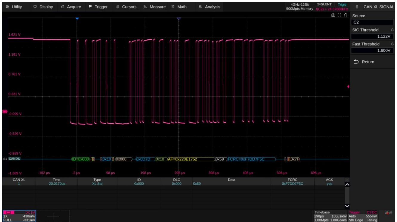
Figure 9 CAN XL SIC Mode Protocol Signal Setting
