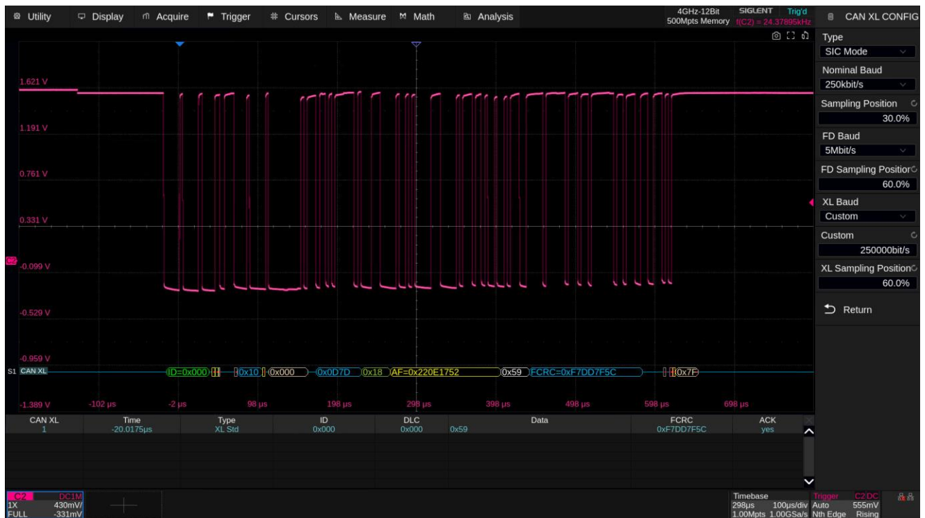
Figure 10 CAN XL SIC Mode Protocol Configuration Settings
