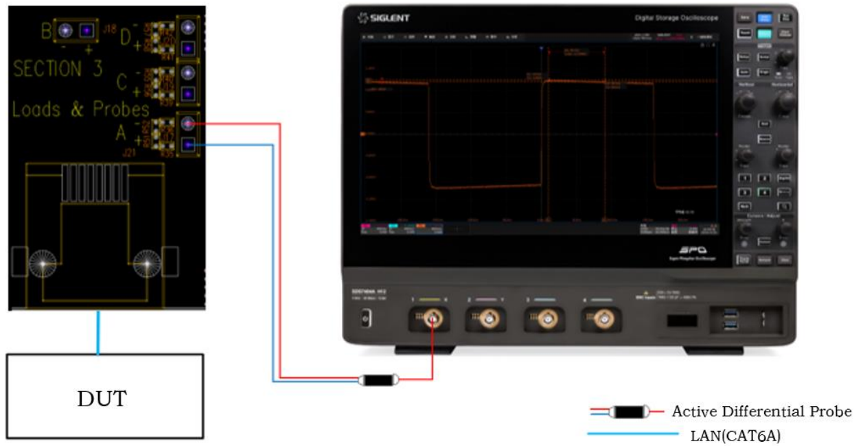
Figure 3-3 Connection Mode of Active Differential Probe
