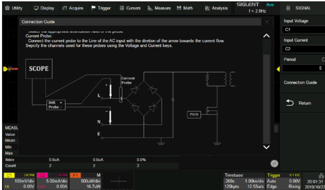
Figure 3: Example of the Connection setup diagram
