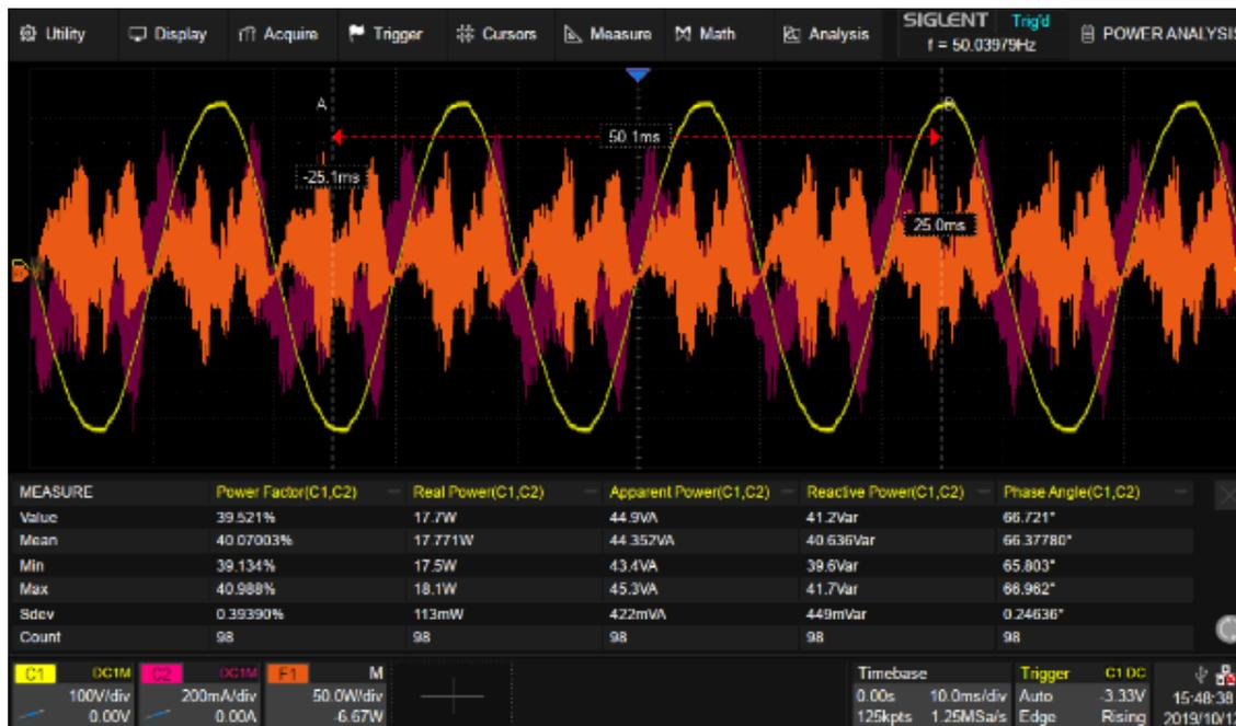
Siglent SDS5000X Power Analysis and Bode Plot function are very convenient and a great time saving option for power circuit engineers.
