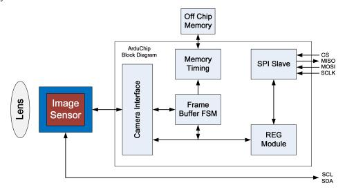
Figure 2 ArduCAM Mini Shield Block Diagram
