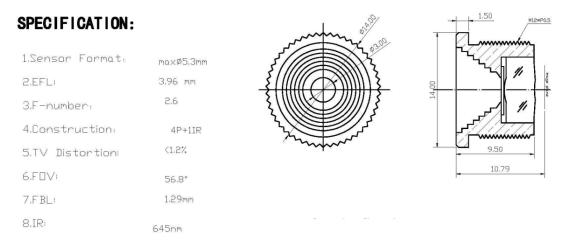
Figure 3 S Mount Lens Specification
