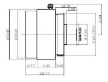
Figure 4 CS Mount Lens Specification
