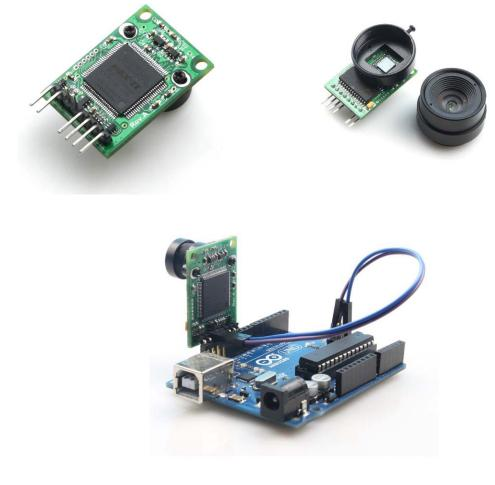
Figure 1 ArduCAM Mini Shield
