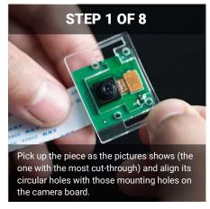
The gap should lie between the left two holes while the white ribbon cable is on the bottom side.
