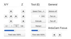
It utilizes these custom commands from your slicer to adjust focus while printing: **@ARDUCAMFOCUSSET <ABS-FOCUS>** to specify an absolute focus. This command is handy to reset the focus when starting a new print after a power failure.
