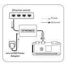
2. Fire TV Ethernet Adapter Mode: Connect an Ethernet cable with network connection to the PoE/Ethernet IN port of this adapter, insert an extra Micro-USB power supply to Micro-USB Power In and then connect Micro-USB Out to your device.
