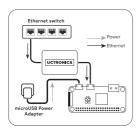
3. Micro-USB Ethernet Adapter Mode: Connect an Ethernet cable with network connection to the PoE/Ethernet IN port of this adapter, and then connect Micro-USB Out to your device. The adapter will not feed power but will deliver Ethernet to your device, which should have been powered with another power supply.
