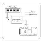
1. **PoE to Micro-USB Adapter Mode**: Use an Ethernet cable running from the Power source (IEEE 802.3af compliant PoE switch or injector) to connect to the **PoE/Ethernet IN** port of this adapter, and then connect **Micro-USB Out** to your device.
