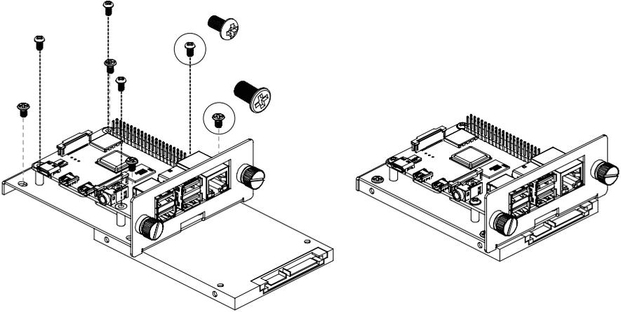
1. Fix the SSD from the back of the bracket with M3\*5 flat head screws first, then secure the Raspberry Pi with M2.5\*5 round head screws.
