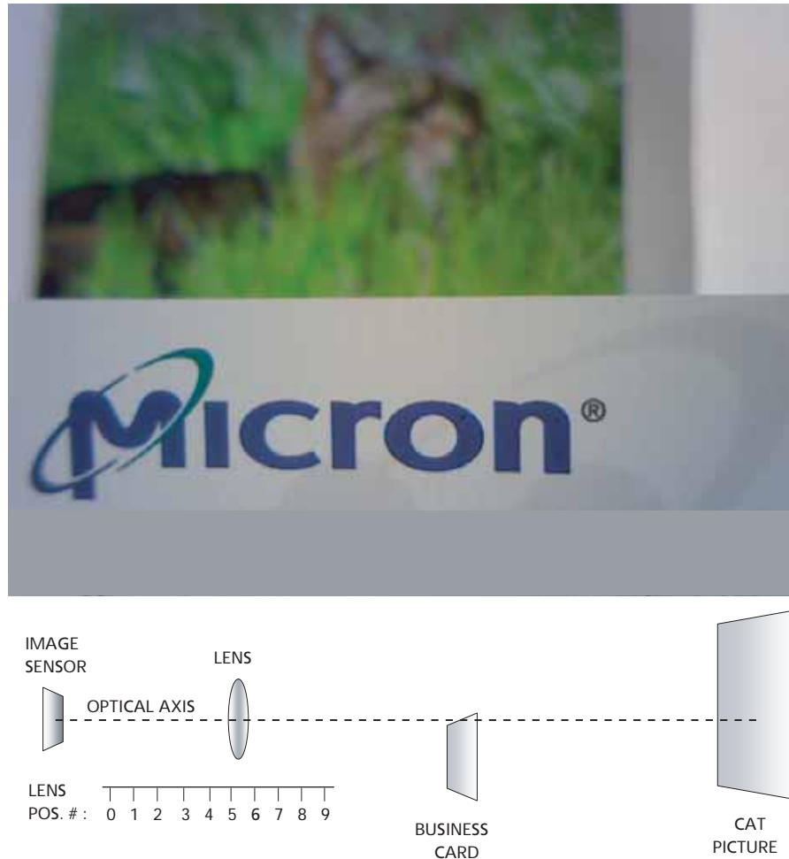
Figure 42: Scene with Two Potential Focus Targets at Different Distances from Camera
