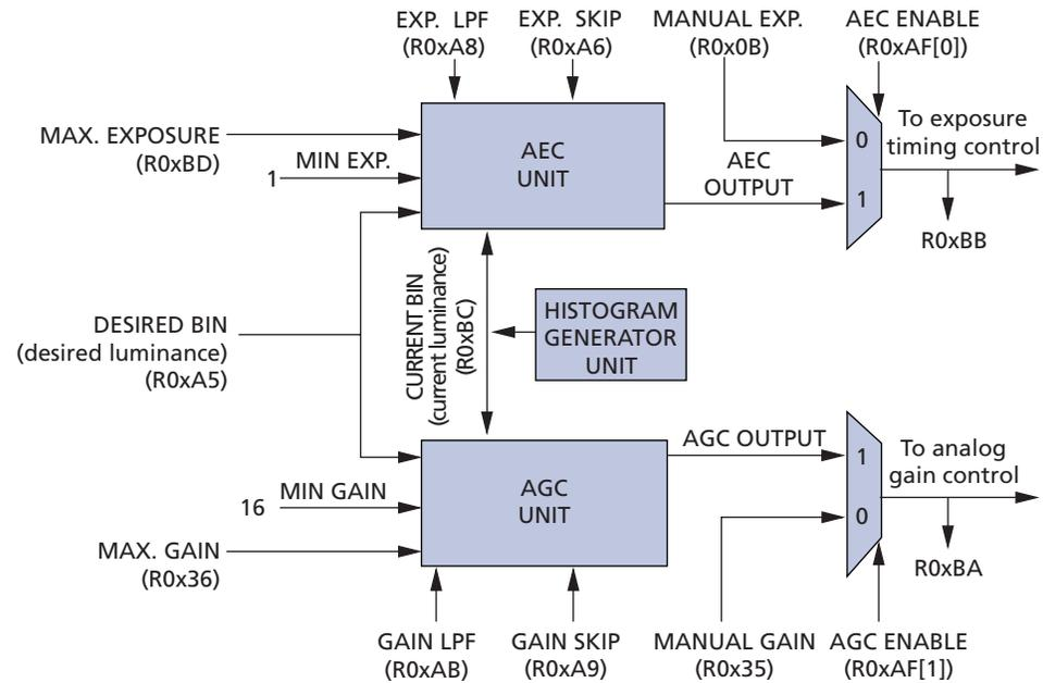
The exposure is measured in row-time by reading R0xBB. The exposure range is 1 to 2047. The gain is measured in gain-units by reading R0xBA. The gain range is 16 to 63 (unity gain = 16 gain-units; multiply by 1/16 to get the true gain).
