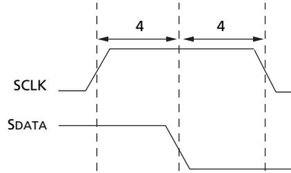
**Figure 38: Serial Host Interface Stop Condition Timing**
