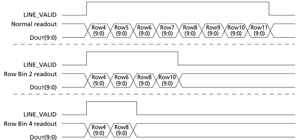
**Figure 31: Readout of 8 Pixels in Normal and Column Bin Output Mode**
