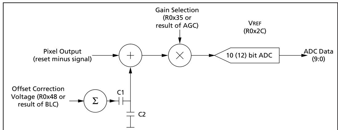
The automatic black level calibration measures the average value of pixels from 2 dark rows (1 dark row if row bin 4 is enabled) of the chip. (The pixels are averaged as if they were light-sensitive and passed through the appropriate gain.)
