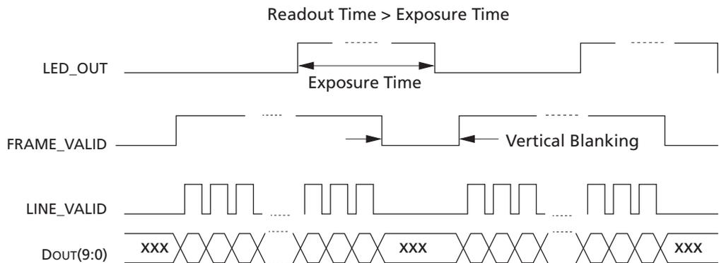
**Figure 14: Simultaneous Master Mode Synchronization Waveforms #2**
